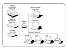
Several GPIB-networked instruments can be connected using the AD007 Adapter to LAN (Ethernet)-based computers and printers.
